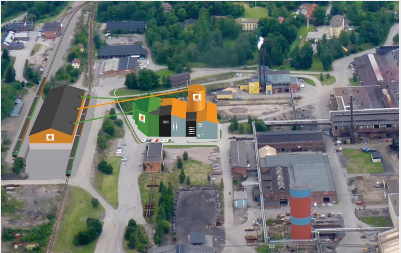
An image of the first FerroSilva plant. Building in a brownfield location has advantages with existing infra structure and services like in Hofors where the closeness to the customer that can take warm DRI directly from the reduction plant is an extra advantage. Layout: Katarina Hamilton.
